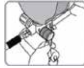
8. Turn Prime/Spray switch to Prime, this will keep storage fluids in sprayer
