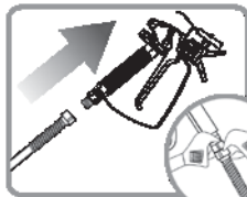
2. Attach and tighten hose to gun.
