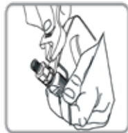
13. Remove trigger guard from housing.
