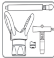
16. Clean all parts in warm soapy water or flushing fluid using a bristle brush.
