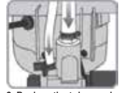
9. Replace the tubes and secure with the clamps
