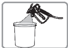
5. Spray into waste bucket until clog clears.
