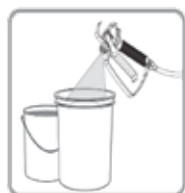
9. Change to waste bucket as paint thins.
