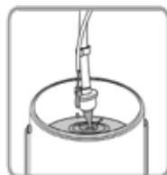
1. Drain paint from tubes
